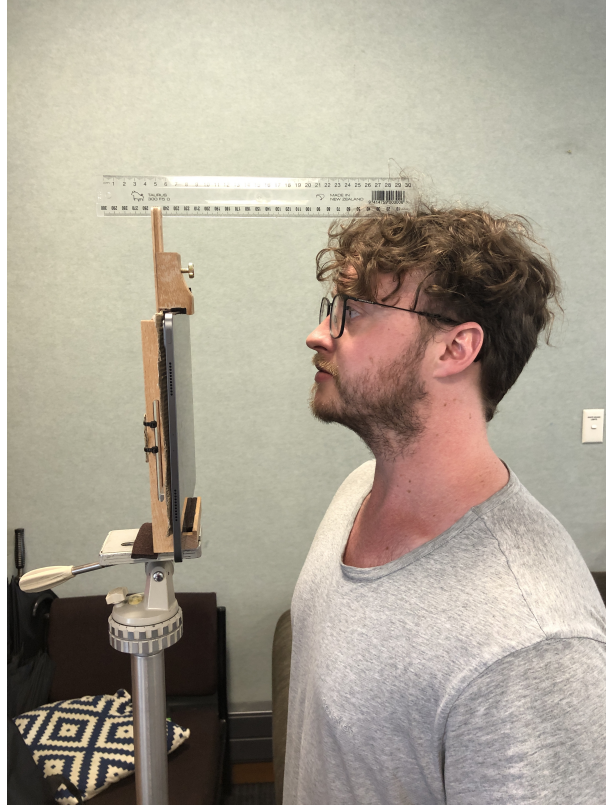
Fig. 2: The vertical orientation. The ruler is aligned with the top of the participant’s head thus placing the surface at the same height relative to the participant. In this case, the individual is an author of the paper.
