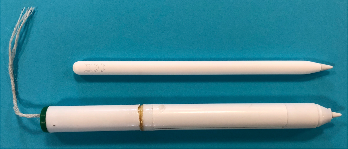
Fig. 1: Apple Pencils in the pen configuration 9 mm x 166 mm (top) and marker configuration 16 mm x 183 mm (bottom).
